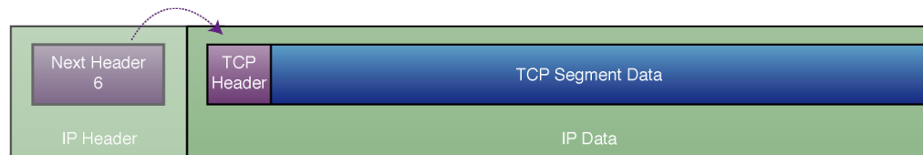
IPv6 Datagram With No Extension Headers Carrying TCP Segment
